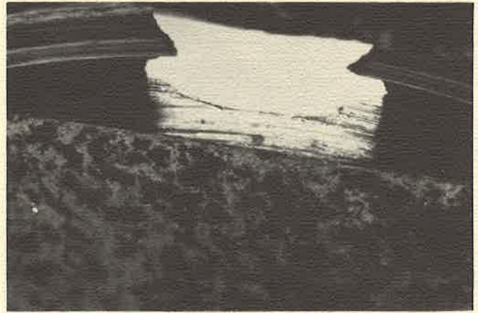
Fig.5 Inside of wheel slot a modern replica pan showing striations made in milling process.
