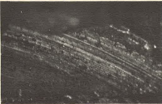
Fig.4 A close-up view of the wheel slot sidewall of an original 17th century wheellock pan. Note the circular and parallel form of the striations left by the wheel when used as a cutter, and compare the shot of the modern pan, made as described in the text. Compare also the small drawing at the corner of the Codex Atlanticus folio , shown in Fig. 8.
