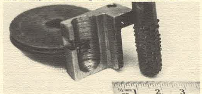
Fig.6 A wheel in its ordinary position in the wheellock pan. The portion of the rim exposed in the pan contains a slanted cross-groove, the triangular walls of which, formed by intersections with the threads of the rim, served as the teeth which milled the slot in the pan for the wheel. To the right is the homemade rasp cutter which cut the powder cavity in the pan.
